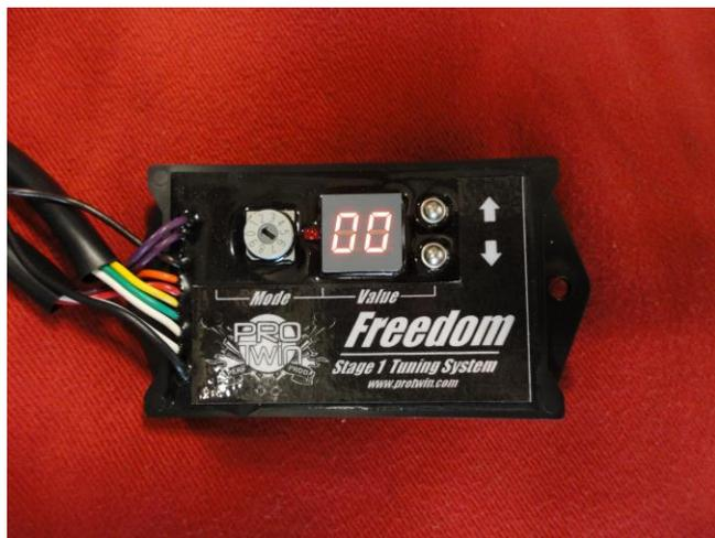
You can use the mode and up/down pushbutton switches to make fuel trim adjustments in the RPM and throttle position ranges required by most applications. The fuel trim value is displayed on a bright daylight readable LED display.
