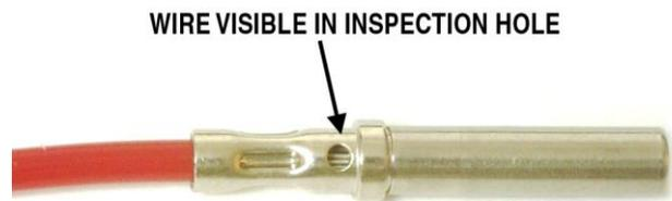
Strip 5/32” insulation from the end of the wire and insert the wire into the terminal as shown in Figure 2. Close the tool to complete the crimping operation. The crimped terminal should appear as shown in Figure 3 with wire strands visible in the inspection hole.
